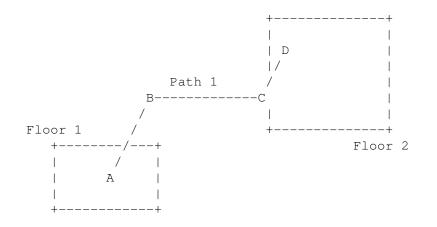
As shown in the diagram, a path can alter direction a number of times. This path has a starting point (A), two "knees" (B and C), and an ending point (D). Up to six point may be defined. Two is the natural minimum.
